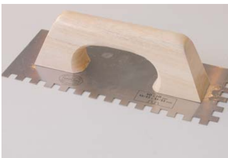
Use a notched trowel.
